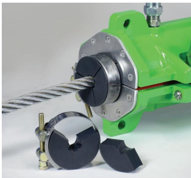
Viper Rope Cleaners enable the removal of contamination or built up old lubricant from the wire rope prior to lubrication, improving the effectiveness of the lubrication process via the Viper WRL. Viper Rope Cleaners (VRC's) are available in left and right hand lay, to suit 6 and 8 strand ropes and other strand configurations on request.
